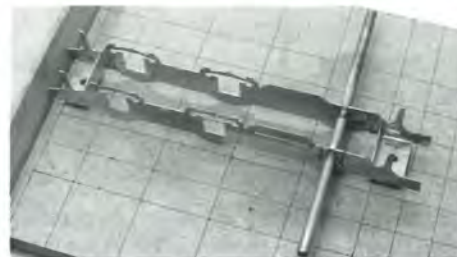
The chassis in course of erection on the fire - spacer tabs located in frames, reference is
