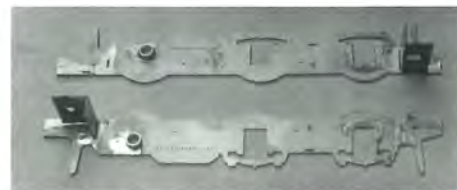
The '57XX' frames ready for final erection, with the two end spacers in place on opposite frame. Note the 'simples' for the rivets on the lower firebox sides, pushed out with a scriber as describe. The bearings of the fixed axle are also in place to act as location for the 'reference rod' during final assembly.
